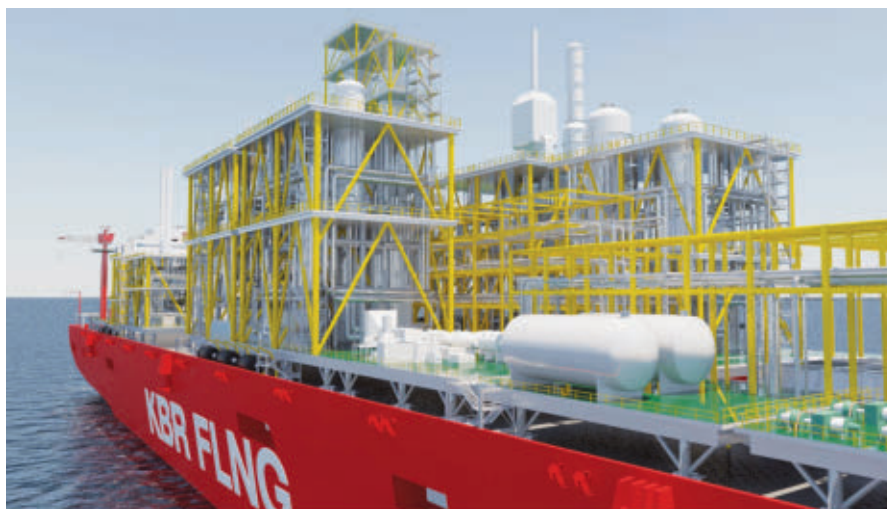
A concept for an FLNG project, showing topsides modules. (All images courtesy KBR)
